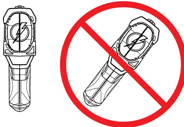
Remember that you can discontinue the discharge at any time by shifting the safety switch to the down (SAFE) position.
